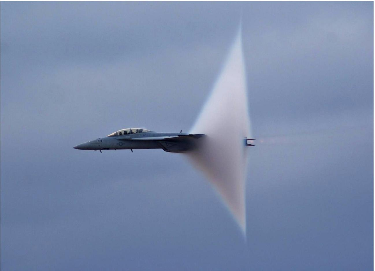
*Fig 33 - F18-Hornet travelling supersonic around which a vapour cone has formed. The air surrounding the jet crosses over from hyperbolic, or supersonic, irrotational flow to subsonic and thus elliptic irrotational flow. The parabolic straight line is seen in the vapour cone.*
